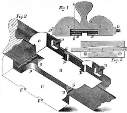
under the weight of the heaviest engine, and the ease with which it can be adapted to old this, too, on an unballasted road bed. The tracks of whatever pattern of rail, recombattering of the ends of the rails, which takes place with most chairs now in use, is effectu- nies. ally prevented by this one, as it renders any considerable working or sinking of the ends of one rail below its fellow impossible. These Small, Esq., Boston, Mass.
