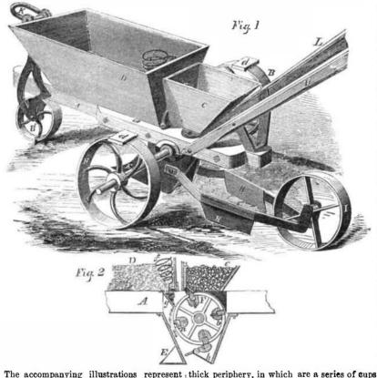
can be regulated to plant different quantities. It deposits guano, or other suitable manure, with the seed, which latter it covers, and then presses down with a roller.
