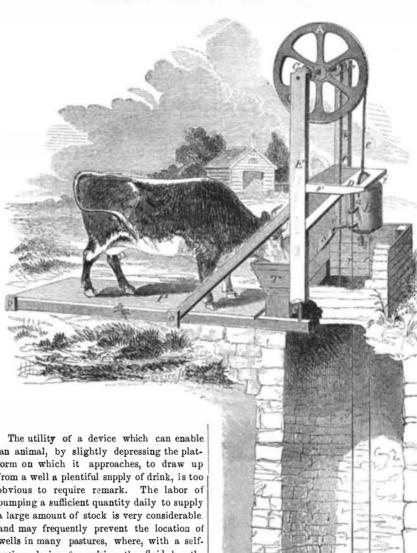
an animal, by slightly depressing the platform on which it approaches, to draw up from a well a plentiful snpply of drink, is too obvious to require remark. The labor of pumping a sufficient quantity daily to supply a large amount of stock is very considerable and may frequently prevent the location of wells in many pastures, where, with a selfacting device for raising the fluid by the weight of the animals themselves, such supplies of water would be highly serviceable.
