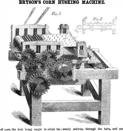
I, is connected at its near extremity to the lever, H, and this lever is actuated by ranning in the oblique groove, g, in the surface of the pulley or cam, J, so as to receive a quick reciprocating motion.
