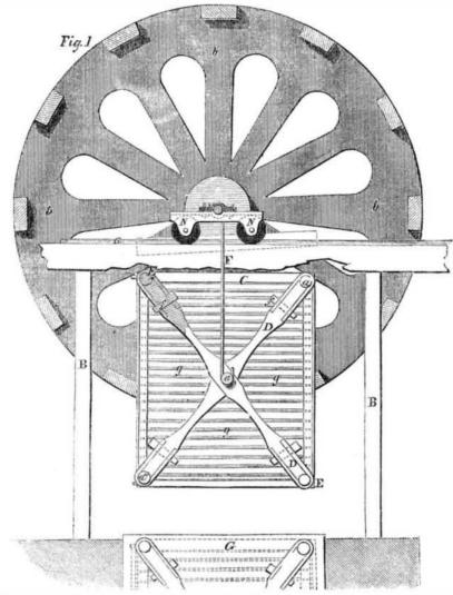
hides bottom side up; and here the special | amined, and if deemed ready the whole is advantage of this arrangement is made appaent. By inserting-a couple of cross bars, one C, and securing to them a couple of hooks attached to the end of ropes wound upon a pair of drums, C. The frame may be raised up out of the vat by turning the large treadwheel, b, secured upon the shaft of the drums.
