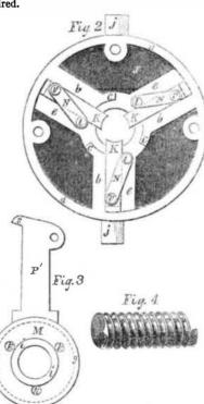
Screws are cut by this machine with great rapidity, and the thread being never of greater size than the plain part, bolts can always be fitted into work perfectly tight, a point of great importance in car or agricultural maas to confine them in their grooves without chine making , bridge building, etc. It is also tool for boring holes of various sizes, the in-
