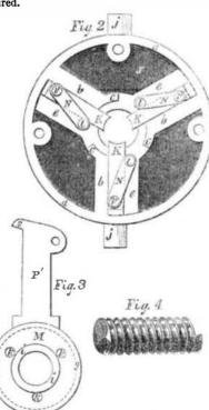
Screws are cut by this machine with great rapidity, and the thread being never of greater size than the plain part, bolts can always be fitted into work perfectly tight, a point of great importance in car or agricultural ma-
