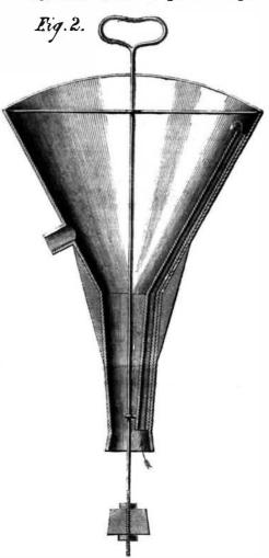
represents another form of the funnel, on the same principle, having an air-tight tube, H, on the inside for the air to escape, other parts being similar. In some cases a metallic screw cone may be used in place of the elastic washer, C, and the nipple, E, be opened and closed in the manner of a spigot working in a faucet, by a rotary motion of the connecting rod and handle, F, and a movable cullender be placed inside for straining liquids.
