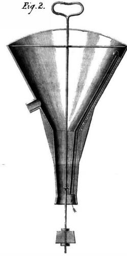
represents another form of the funnel, on the same principle, having an air-tight tube, H, on the inside for the air to escape, other parts being similar. In some cases a metallic screw cone may be used in place of the elastic washer, C, and the nipple, E, be opened and closed in the manner of a spigot working in a faucet, by a rotary motion of the connecting rod and handle, F, and a movable cullender be placed inside for straining liquids.
