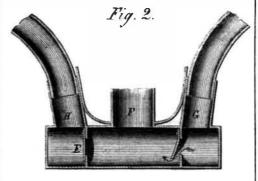
valve, H, thus rendering exhalation and inhalation comparatively free, and separating pure from foul air. This device would be useful in foul wells where carbonic acid gas collects in cess pools, or in similar places.
