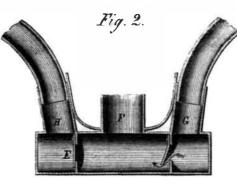
valve, H, thus rendering exhalation and inhalation comparatively free, and separating pure from foul air. This device would be useful in foul wells where carbonic acid gas collects in cess pools, or in similar places.
