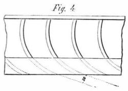
the wheel is at work and filling the step chamber, bears up against the diaphragm, D, and finally escapes at the inside edge of the chamber. This does not in any way affect the discharge which takes place at the bottom of the buckets.
