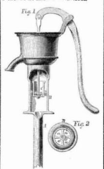
When the plunger, C, is forced down, the valves, a a, open, and the water flows up; when raised, the valves close, and the plunger then lifts the water. The elastic ring packing is kept in place by the form of the outside of the plunger, and it can roll up and down with the motion of the plunger, and maintain its position always air-tight. Being elastic, it accommodates itself to any roughness or inquire to be turned in a lathe.
