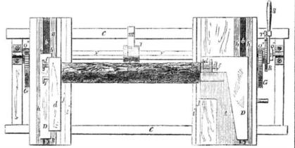
provement in combining and operating the slides of the blocks of a saw mill, whereby with one motion of the lever the two slides are moved with ease, simultaneously to feed the log the exact and equal distance tranverse-
