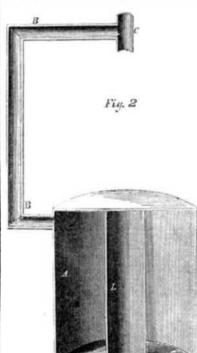
d, of the top fig. 3 is then secured air-tight to the top of jar K, by means of the cement which adheres to glass and tin (and will not melt at the temperature of boiling water.) The jar being filled with fruit, as shown in fig. 1, and the top being placed in its position, and the cement in the groove for its reception being cooled, the tube G, (figure 3,) and tube C, (figure 2,) are connected together, the pipe, C, slid over G, and cement-
