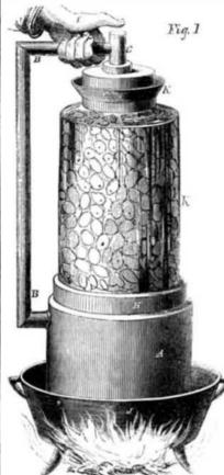
after the expulsion of air. The tin tube, B, is soldered to the side of the can and the tube. d, is made to fit smoothly in the jar, K, intended to be used. The flange, D, flared at top and narrow at its bottom, is for holding cement. The space that is left between the two tubes, F and G, is for the introduction of melted cement. In the center of the top, E being also in the center of tube G, is a small hole of one-eighth of an inch in diameter.
