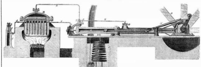
the vapor is alternately conducted first to one cylinder and then to the other, pushing forward first one piston and then the other. At the return stroke of each piston, the gas escapes by an exit port, as in an ordinary steam engine, and is conducted by a pipe, b, to the condenser, where its elastic force is destroyed, and it is reconverted into a liquid.
