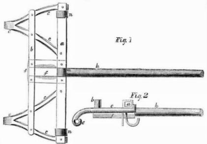
The accompanying figures represent an im provement whereby a carriage can be readily adapted for one or two horses, by attaching a frame to the running gear, by clips, and providing sockets for the reception of a pole, and
