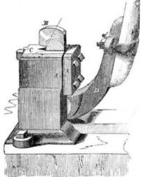
The arrangement of the dies in this machine avoids all trembling or vibratory motion, rendering this machine equally adapted to gumming or cutting the teeth of mill, crosscut, circular, and other saws-giving the operator the privilege of alternately changing the saw, and also of cutting the teeth of any desirable shape without straining or twisting
