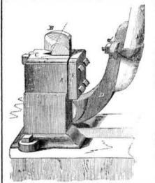
The arrangement of the dies in this machine avoids all trembling or vibratory motion, rendering this machine equally adapted to gumming or cutting the teeth of mill, crosscut, circular, and other saws-giving the operator the privilege of alternately changing the saw, and also of cutting the teeth of any desirable shape without straining or twisting the saw.
