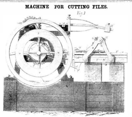
gears with the wheel, V, on the shaft, E, and fixed on two peg wheels, 1 and 6, which gear on either side with intermediate wheels, 2, 3 4, and 5. A spring above and one beloweach hammer handle regulate the force of the blows.
