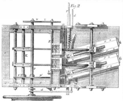
cut with double cross cuts. The inclination of the cuttings of the file is given by the inclination of the carriages, FF. The wheel, W, on the shaft outside the frame gears with the wheel, V, fixed on the same shaft as the
