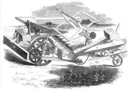
Manny's improved Harvester, embracing the machine for farmers. It has now been deresult of several patents—two being granted on the 21st of October last. These two cover improvements in preventing the cutters from choking; also in preserving them horizontally, while the finger also conforms to the inequalities of the ground. Anoter, granted on the 4th of last month, relates to an improvement in the raking operation.
