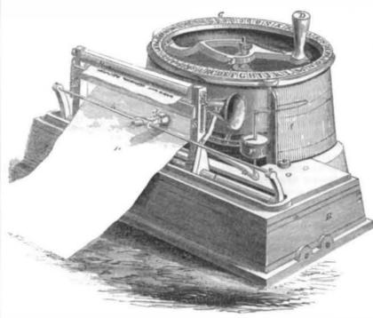
mechanism for moving the paper is very sim ported on, and revolves on anti-friction rollers underneath, so that the operation of working it is very free and easy.
