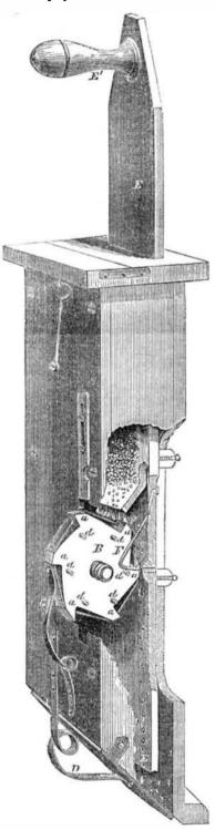
The periphery of wheel B is notched at intervals, so as to form pockets, a, which receive the seed. By the revolution of wheel B, the seed contained in said pockets is discharged, and falls to the lower part of the machine, below slide E, upon the plate C; this plate is hinged at c, but is kept closed, except at the moment of planting, by the spring D.
