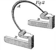
This is an economical device. This kind of fastening may also be applied to the man-hole covers of boilers. The patentee, John G. Hock, of Newark, N. J., has also taken out patents in Europe for this invention, and also for an improvement in Gas Retort Benches. Being engaged in the business of manufacturing illuminating gas, he is well acquainted with the defects of common apparatuses, and knows what improvements are required.
