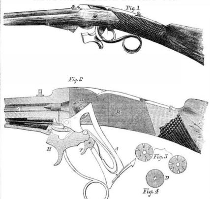
arm A, is thrown out of catch, and drawn This is a valuable improvement in breechdown to the position shown in figure 2, by its loading arms, allowing them to be loaded with swinging on its swivel or axis pin; the car- great ease and rapidity; and all the parts are tridge is now thrust in, as shown, the arm simple, and not liable to get out of order. pushed up again, when it locks itself, and it acts of pulling down and up the arm, A. Albany, N.Y.
