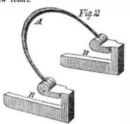
This is an economical device. This kind of fastening may also be applied to the man-hole covers of boilers. The patentee, John G. Hock, of Newark, N. J., has also taken out patents in Europe for this invention, and also for an improvement in Gas Retort Benches. Being engaged in the business of manufacturing illuminating gas, he is well acquainted with the defects of common apparatuses, and knows what improvements are required.
