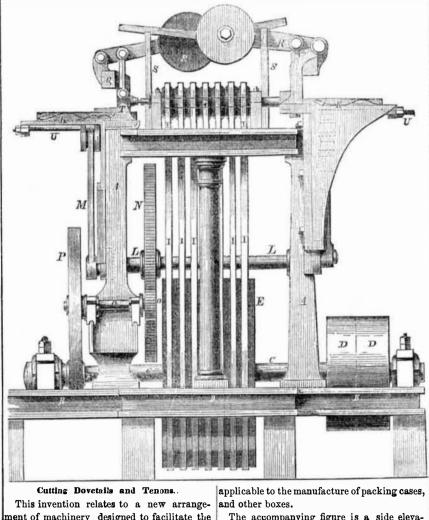
MACHINE FOR CUTTING DOVETAILS AND TENONS.
