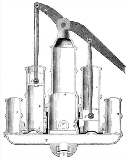
tailing experiments which had been made | - "The application of the air chambers, B B, with and without such vessels. A very large to the supply pipes or engines, together with increase of duty was obtained by the use of the manner in which the pump is cast, as these air chambers. The usefulness of air shown and described." chambers connected with the supply pipes of pumps is now generally admitted, but as we stated before, few are aware of the existence of this extended patent relating to them.
