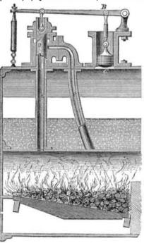
steam-tight piston, having metallic packings, the piston being exposed to the action of the steam. The top of the piston is pressed down by springs giving a resistance of 80 lbs. per inch. Connected with the piston is a valve, D, for the admission of water from the boiler on to the fire. When the piston is pressed upwards, the valve, D, moves upwards through three times the space of the piston, and by this means opens the communication, F, between the beiler and for water.
