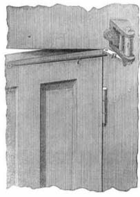
Another advantage of this arrangement is that the travel of the spring is essentially lessened, in consequence of the crank arm being made to turn inward when the door is opened. The necessity of its being strained to an undue degree when the door is opened wide is thereby almost entirely obviated. The durability of the spring is thus increased very much. The whole travel of the spring is about one-eighth of a turn.
