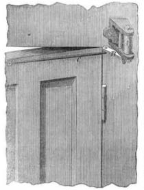
Another advantage of this arrangement is that the travel of the spring is essentially lessened, in consequence of the crank arm being made to turn inward when the door is opened. The necessity of its being strained to an undue degree when the door is opened wide is thereby almost entirely obviated. The durability of the spring is thus increased very much. The whole travel of the spring is about one-eighth of a turn.
