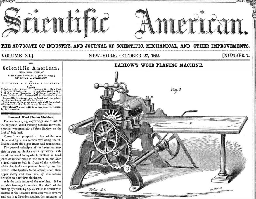
greater or less, according to the surplus wood from the rollers, its upper side rests against the feeding force. bearing plate, b, with a considerable pressure, because the weight of the plank acts upon the inclined position of the plate. This prevents
