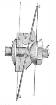
This is a most ingenious contrivance, and will save the great expense of having saws made to the thickness of the rebate required. The invention has been patented by Mr. Henry Laxton, as a communication from feet, and is then parched or dried in the sun Messrs. Highfield and Harrison, of the United
