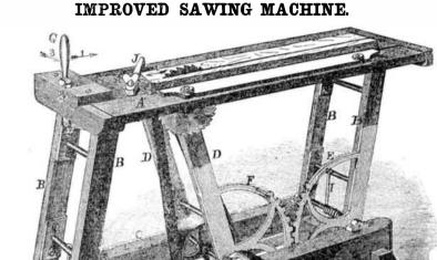
make it vibrate easily. J is a quadrant gauge | any place, and can be set up in a few minutes. attached to the table for mitering. When not The parts are quite simple. It can be altered wanted, it may be quickly removed, by unscrewing its thumb button.
