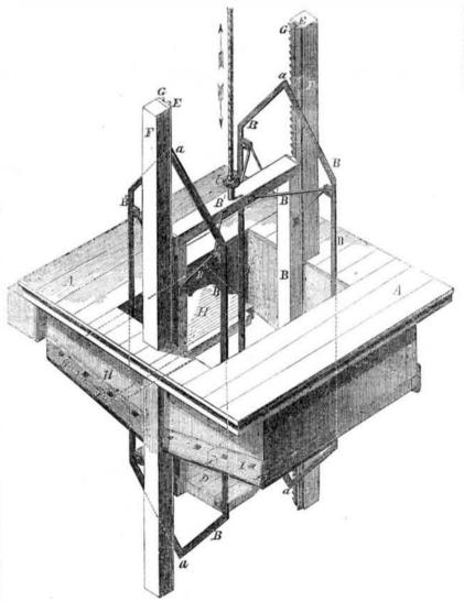
improved Safety Hatch, adapted to eleva- posts, F. G are ratchet toothed racks, so contors, for the use of mills and warehouses, for nected by pawls with the rope, that in case which Letters Patent were granted to William | the rope should break, the pawls are instantly H. Thompson and Eustis P. Morgan, of Biddeford, Me., June 24th, 1856.
