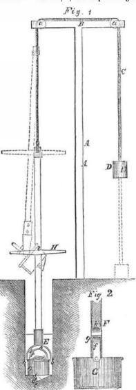
in its proper position. H is a handle on the shank or pole, E, said handle being allowed to move up and down on the shank or pole, and prevented from turning upon it by a key, i.
