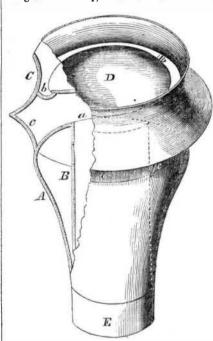
egress. Thr upper part, C, of the cap is made of sheet iron, and is somewhat larger in diameter than the largest part of A. This part, C, is made flaring both ways, as shown, and to its inside is attached a disk, D, which is larger than the orifice, a. This disk is sustained by braces, b b. The flaring cap, C, is sustained by braces, cc, as shown. It is now ready for being attached to a chimney by its lower end, E, which is substantially secured in position
