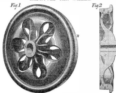
tions in the other one, so that any fracture its superiority. would have either to pass through the wide part of one of the flanges, or to run obliquely across the tread of the wheel.
