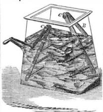
The invention consists in the employment of two swinging dashers, A A', which are suspended from pivots, C, within the churn and work in opposite directions. The beaters, E, of one dasher passing between the beaters of the others, whereby the cream is subjected to the requisite agitation or commotion, so as to produce butter in the shortest possible time, and with but a small expenditure of power.
