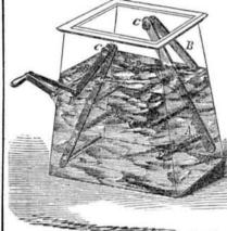
The invention consists in the employment of two swinging dashers, A A', which are suspended from pivots, C, within the churn and work in opposite directions. The beaters, E, of one dasher passing between the beaters of the others, whereby the cream is subjected to the requisite agitation or commotion, so as to produce butter in the shortest possible time, and with but a small expenditure of power.
