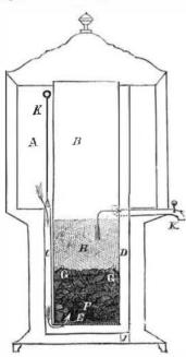
This invention is adapted to the filtering of water on a large as well as a small scale. It may be made in the form of a cistern, and sunk in the ground. In such cases the water from the eaves spouts is conducted to chamber A, and is raised by a pump from chamber B. The filter is cleansed by the application of a pump to the upper end of the tube, D. The water in B will thus be drawn down through the filtering materials, bringing away the impurities and discharging them through D.
