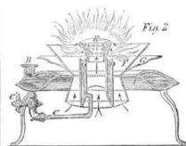
air passes up through the burner into the cone and escapes, through the perforations, into the flame, thus increasing the supply of oxygen, causing most perfect combustion, and augmenting the intensity of the heat. F G are reflectors, which throw the heat upwards into the oven and increase the temperature in that
