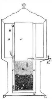
water on a large as well as a small scale. It may be made in the form of a cistern, and sunk in the ground. In such cases the water from previously used—and these patents are fully the eaves spouts is conducted to chamber A, and is raised by a pump from chamber B. The filter is cleansed by the application of a pump to the upper end of the tube, D. The water in B will thus be drawn down through the filtering materials, bringing away the impurities and discharging them through D.
