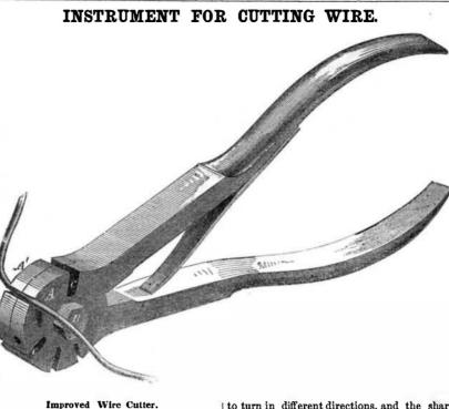
When wire is cut by means of the common nippers, or bent back and forth with plyers until it breaks, there is a burr left upon the pieces, which must be placed in a vise or smoothed off with a file. The wire must also be straightened out again by hand. These inconveniences, although not amounting to much individually, become very objectionable where any considerable quantity of wire is to be cut, or nice work desired, as for example in pianoforte making.
