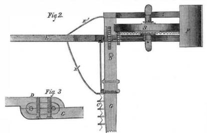
chine is rendered very compact. The method, dressing Messrs. Buckmaster & Wise, as above, of constructing the frame and attaching the who are jo nt owners and extensive manufactongue is at once simple, strong, and economical in construction. The joint between bars D and G is also cheap, but very strong. This invention possesses several valuable features, and will, no doubt, find favor among agriculturists.
