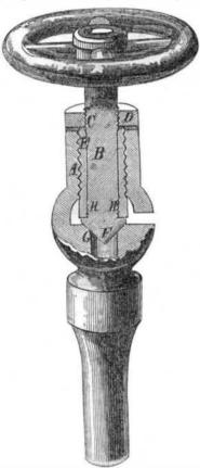
Referring to the above engraving, the improvement consists in having an outer shell, E, shipped over the spindle, B, and fastened as shown, at the screw threads, H H, and further secured by a flat nut, D, screwed hard against the end of shell E, at the thread, C. By turning back the hand wheel, the valve, F, is opened, or run back from the seat, G, allowing the steam or water to pass out through the opening below; the part, I, should be six-sided.
