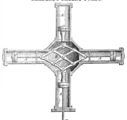
inlet valve, and on its cover an outlet valve. ber, B, when forced inwardly will discharge C C, by the action of the cross levers. The
