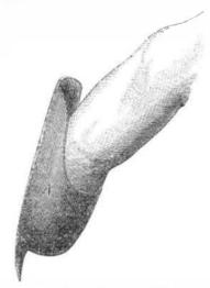
The present improvement consists of a thimble, A, the bottom part of which is furnished with a small cutter, B. The thimble is worn upon the finger and used in place of the nail. It is an effectual remedy for the evil above mentioned.
