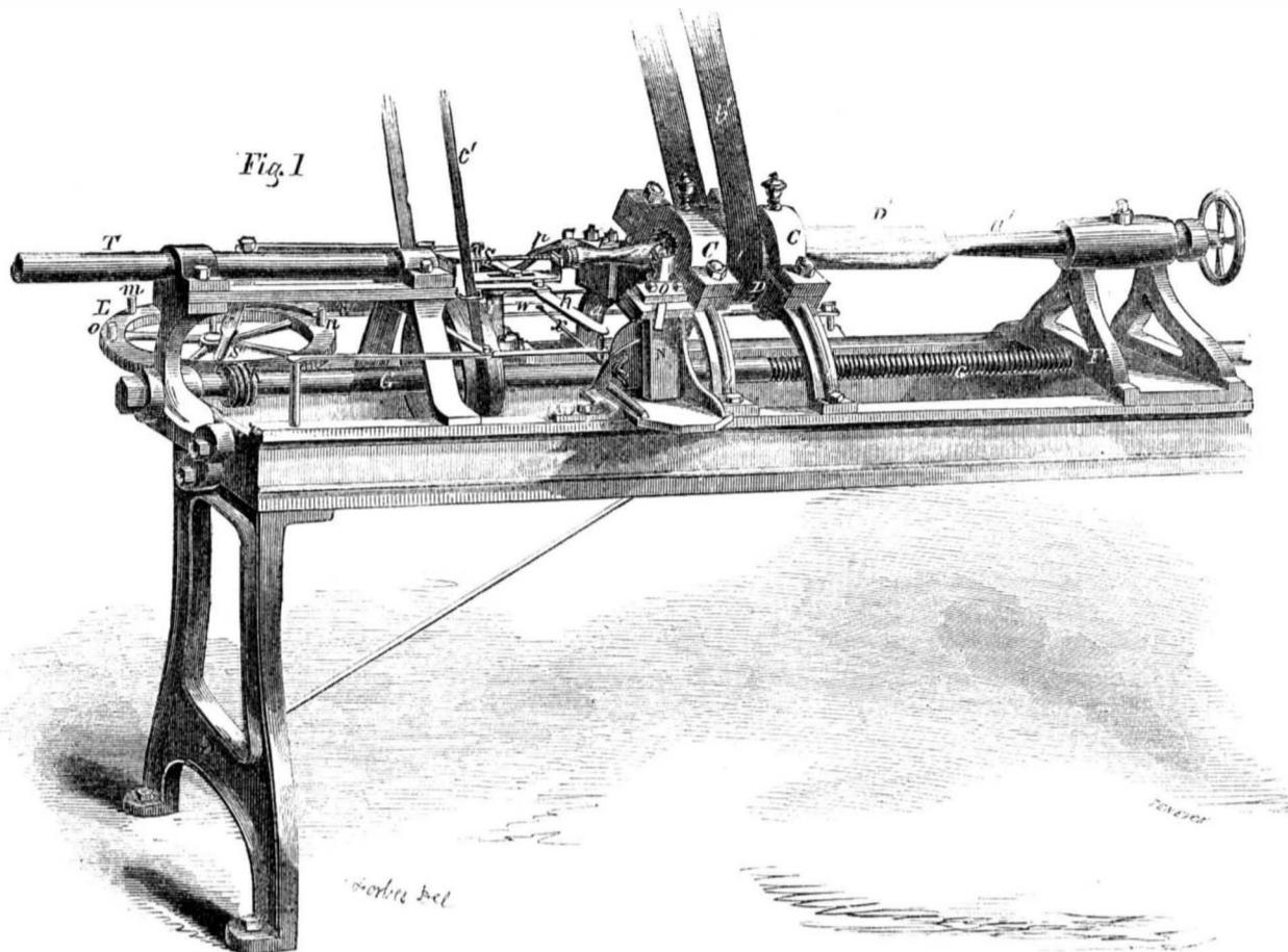
which throws off the belt, c, and stops the feed screw, G, the instant that a given pattern is finished.
