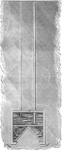
In our engraving, A is the cistern, which is open at the bottom and divided within by diaphragms, or partitions, A', B B'. The water rises through perforated diaphragm, A', into reservoir C, whence it is made to ascend through pipe D, by means of the pump. E is an air pipe extending from the surface of the ground to the reservoir.
