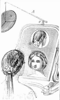
nary toilet glass by means of a thumb screw C, and when the rod is drawn out in the position shown in the drawing, the back of the head is at once reflected in the glass; when not required for use the circular mirror can easily be placed back at the top of the glass out of the way, so as not in the least to interfere with the ordinary use of the glass. This is an ingenious contrivance. Exhibited at the late exhibition of the Society of Arts and Manufactures, London, by Messrs. Heal &
