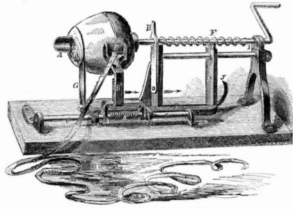
Apple Parer, Corer, and Slicer. holder, A, and revolved by means of the crank. force of spring J is now sufficient to push E' The paring knife, B, is mounted on a standard, B', which slides on rod C. Standard B' is connected by means of brackets, D, with slide, E, the upright of which, E', is forked, so as to mesh with the wire screw thread, F. G is the slicing knife standing upright, and attached to one end of E.
