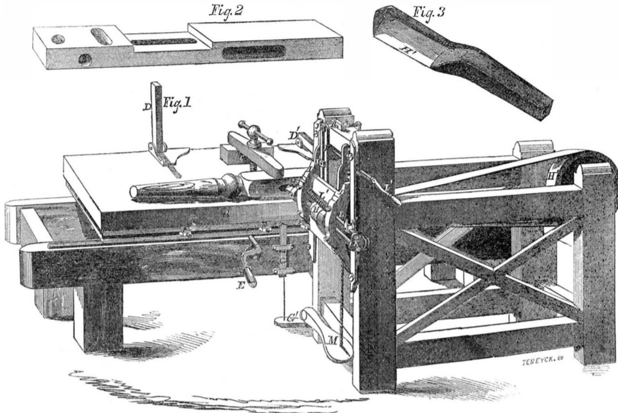
of stuff, such as bed posts, car frames, &c., all exactly alike, without new adjustment for each. The cutter makes clean and finished work. Any desired number of studs, F, may be introduced on the bed, B, and the number of slots to be mortised in the stuff increased
